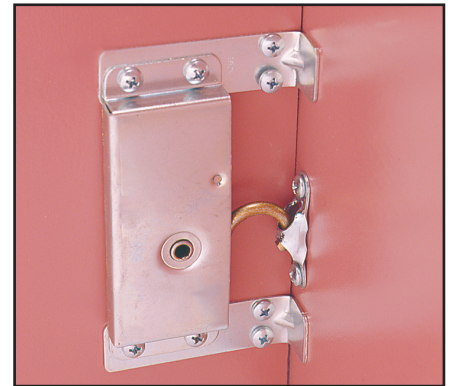
Fig. 8C Type 1R Latch with braces and 'U' Receiver for holding inside corners tight and at 90°. (See TDS 40)
