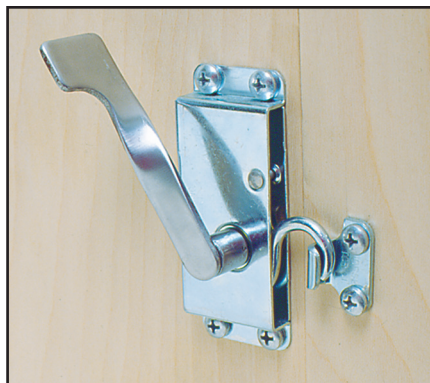
Fig. 12 Type 1R Latch with handle and a 'J' Receiver for a 'same plane' surface mounted application. (See TDSs 37 & 39)
