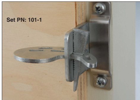
Fig. 1 PLYWOOD IS CLAMPED DOWN AGAINST WINDOW FRAME FACE. HARDWARE MOUNTS ON FRAME FACE. A PERMANENT "KEEPER" IS USED. SEE TDS 206-2A.
