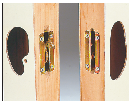
Fig. 6 (Re: Fig. 5) Unlocked in-line butt joint using a Type 3 Latch and Receiver flange-to-flange in this cut-away view. This is the most frequently used Norse Latch/Receiver combination for exhibit fabrication. (See TDS 108)
